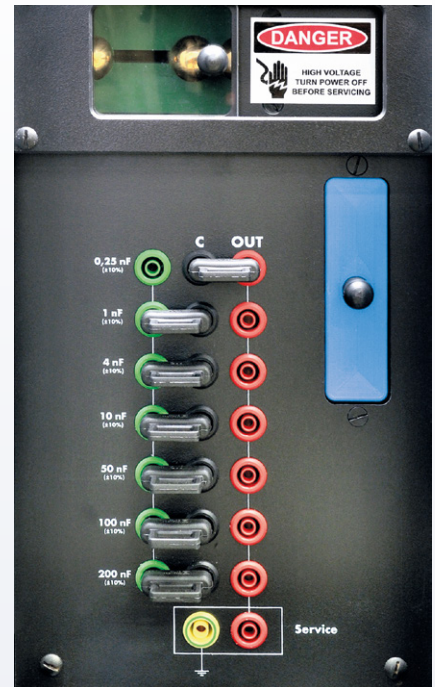
Capacitor selector switchboard
