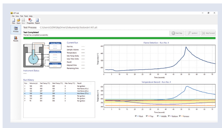
AIT-Lab software – measurement of auto-ignition temperature
